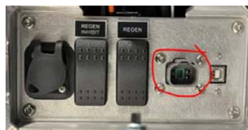
V-MUX connector may be a pigtail or mounted as above
