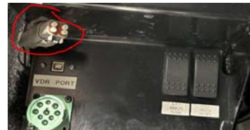
V-MUX connector may be a pigtail or mounted as above
