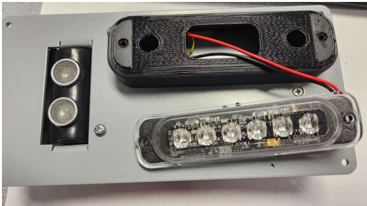
Figure 11: TWS adapter placed and installed to faceplate
