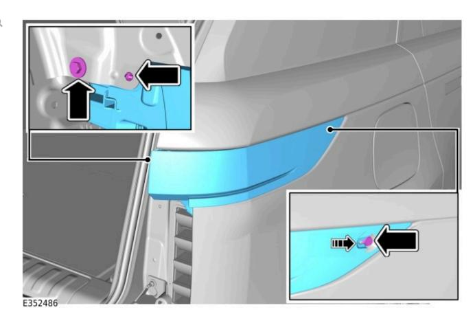
• Install the rear right lamp assembly electrical connector to the clip.
