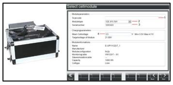
Follow the VAS6910 operating instructions in conjunction with the DSS Manager program to perform the cell balancing on the new cell module.
