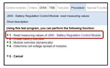
Select the option "Read measuring values of J840 – Battery Regulation Control Module."
