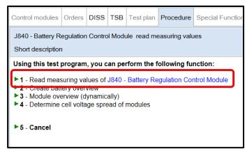
Select the option "Read measuring values of J840 – Battery Regulation Control Module."
