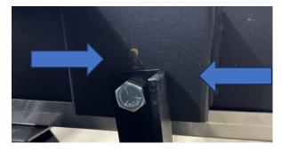
If cracking is present in the hat bracket, remove it by cutting the welds and welding in a new hat bracket. Part number 455556-3.
