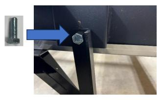
After the new bracket has been installed, and the bolts have been replaced, the spare tire can be placed back into the carrier.
