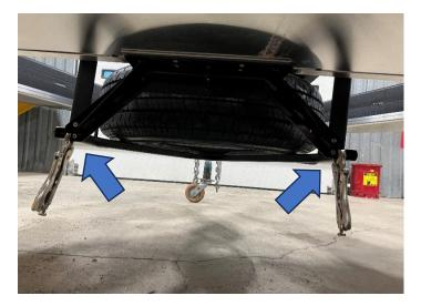
Using a drill with a #11 (3/16") drill bit, drill out the holes in the top of the bracket and the arms. Use a pop gun to install stainless rivets (part # 330031-03) 2 in each arm, 4 on the bottom side of the bracket, and 6 on the top side of the bracket.
