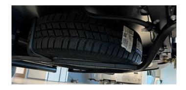
Before installing the new spare tire carrier bracket the original hat bracket needs to be inspected for cracking. If any cracking is present, the hat bracket will need to be replaced.
