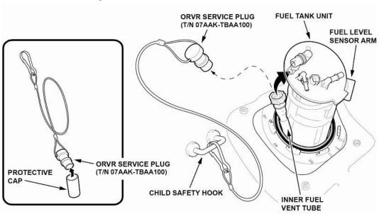
56. Remove the ORVR service plug from the child safety seat hook, and install the provided protective cap.
