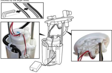
51. While compressing the fuel tank unit, make sure the movement is smooth and the fuel tube and wiring harness do not stretch, pinch, or bind.
