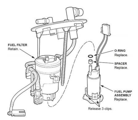
43. Install the new spacer onto the new fuel pump motor.
