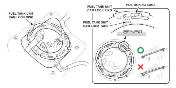
60. Tighten the fuel tank unit cam lock ring by turning clockwise using the fuel sender wrench.
