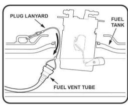
34. Remove the fuel tank unit with the O-ring.
