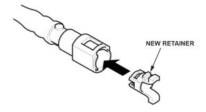
62. Connect the fuel line quick-connect fitting and connector.
