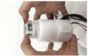
47. Install the fuel filter assembly to the reservoir.
