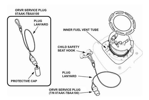
31. Disconnect the inner fuel vent tube from the fuel tank unit, and hold it.
