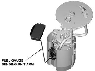
12. Unlock the fuel tank unit cam lock ring.
