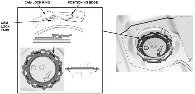
17. Using the fuel sender wrench, turn the fuel tank unit cam lock ring clockwise.
