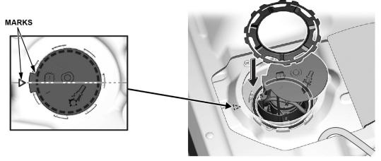
16. Rotate the fuel tank unit cam lock ring and slide the fuel tank unit cam lock tabs into the positioning edge slightly as shown by hand.
