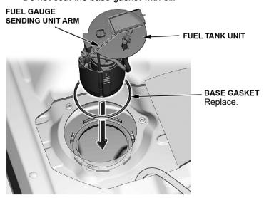
15. Align the tab of the fuel tank unit and the marks on the fuel tank, then insert the fuel tank unit into the fuel tank.
