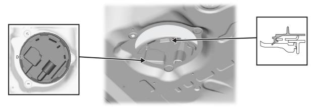
19. Connect the fuel feed quick-connect fitting to the fuel pump; make sure you can hear a click sound.
