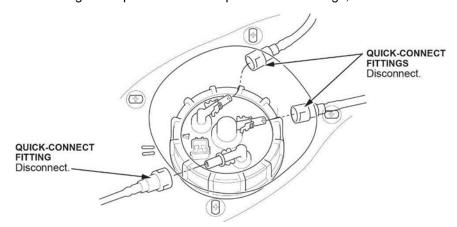
21. Loosen the fuel tank unit locknut using the Fuel Sender Wrench (T/N 07AAA-S0XA100).
