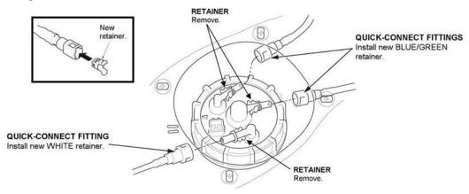
47. Connect the quick-connect fittings to the fuel tank unit.
