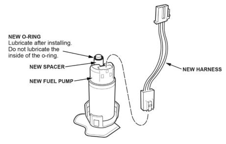
35. With the palm of your hand press the fuel pump into the suction fuel filter.
