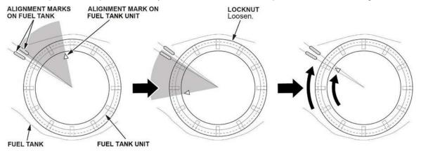
46. Remove the quick-connect fitting retainers on the fuel tank unit, then install the new retainers to the quick-connect fittings as shown.
