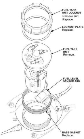
23. Prepare the fuel tank unit and parts to be replaced.
