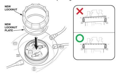
44. Tighten the fuel tank unit locknut to the specified torque using the fuel sender wrench.
