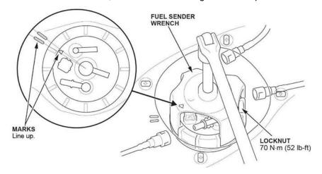
45. If the marks do not line up, friction between the fuel tank unit and the locknut may cause the fuel tank unit to turn while tightening. Observe the difference (shaded area) and loosen the locknut until the fuel tank unit can be rotated. Rotate the fuel tank unit counterclockwise by the same amount and repeat the tightening process.
