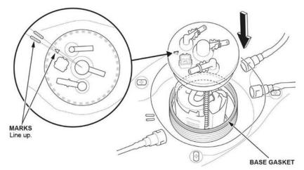
43. Hold the fuel tank unit vertically and tighten the new fuel tank unit locknut with a new locknut plate by hand.
