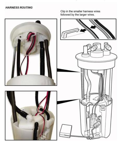
40. While compressing the fuel tank unit, make sure the movement is smooth and the fuel tube and wiring harness do not stretch, pinch, or bind.
