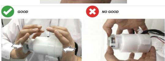
36. Install the fuel filter assembly to the reservoir.
