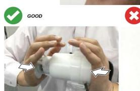
27. Install the fuel filter assembly to the reservoir.
