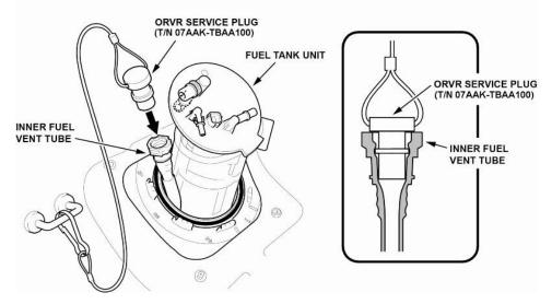
32. Install the ORVR service plug to the inner fuel vent tube. Make sure the ORVR service plug is fully seated by holding the inner fuel vent tube and gently pulling on the plug's lanyard.
