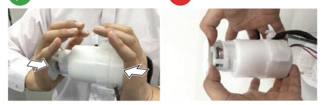
47. Install the fuel filter assembly to the reservoir.
