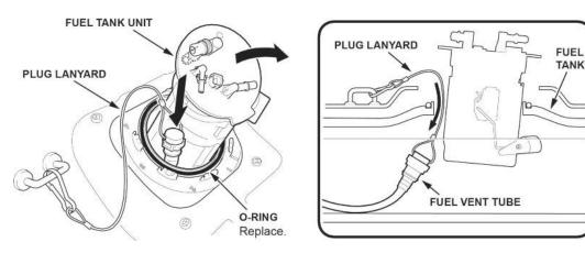
34. Remove the fuel tank unit with the O-ring.
