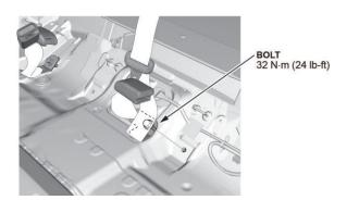
18. Remove the fuel tank unit access panel, and disconnect the connector.
