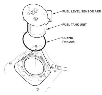
35. Prepare the fuel tank unit and parts to be replaced.
