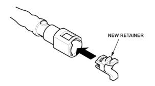
62. Connect the fuel line quick-connect fitting and connector. NOTE: Install the connector cover if it was removed.
