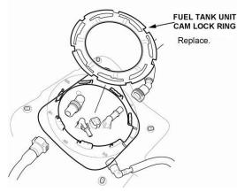
29. Partially remove the fuel tank unit.
