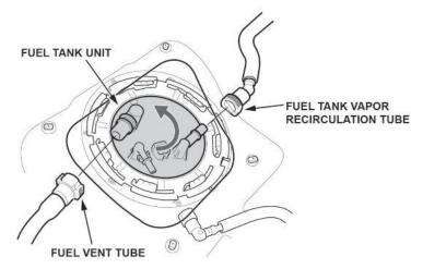
59. Turn the fuel tank unit cam lock ring by hand, and slide the fuel tank unit cam lock tabs to the positioning edge as shown.
