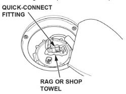
18. Disconnect the quick-connect fitting from the fuel tank unit.
