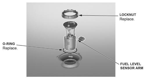
21. Prepare the fuel tank unit and parts to be replaced.
