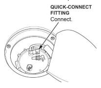
46. Connect the fuel tank unit connector.
