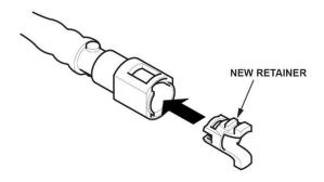
45. Connect the fuel line quick-connect fitting.
