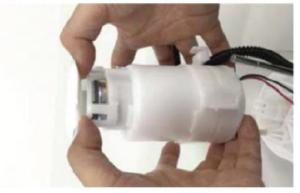
33. Install the fuel filter assembly to the reservoir.
