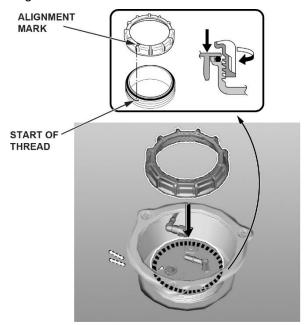
41. Press down on the fuel tank unit while turning the locknut clockwise by hand.
