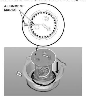
40. Align the mark on the new locknut to the start of the thread on the fuel tank.
