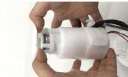
17. Install the fuel filter assembly to the reservoir.
