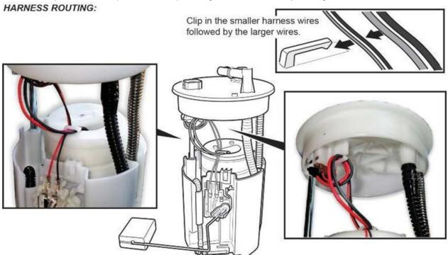
21. While compressing the fuel tank unit, make sure the movement is smooth and the fuel tube and wiring harness do not pinch or bind.
