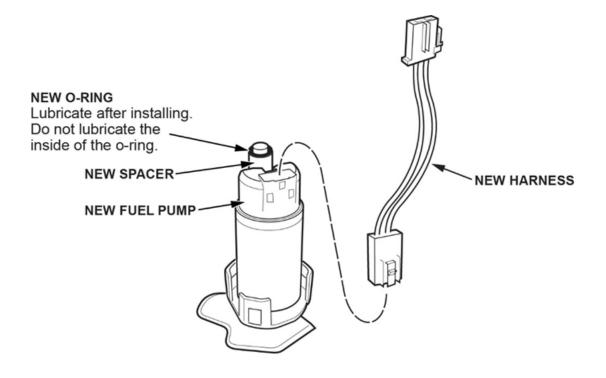
39. With the palm of your hand press the fuel pump into the suction fuel filter.
