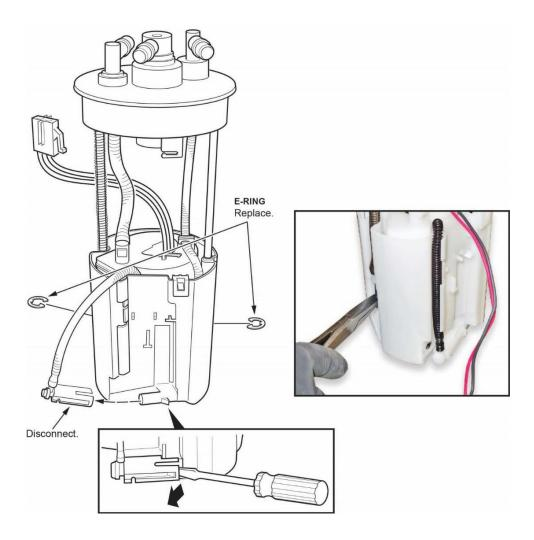
32. Disconnect the joint at the bottom of the reservoir.
