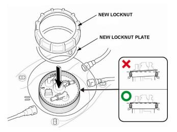
47. Tighten the fuel tank unit locknut to the specified torque using the fuel sender wrench.
