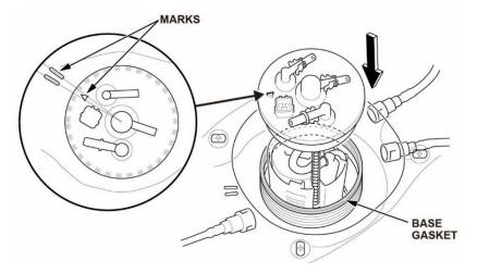
46. Hold the fuel tank unit vertically, and tighten the new fuel tank unit locknut with a new locknut plate by hand.
