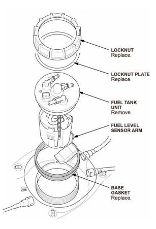
27. Prepare the fuel tank unit and parts to be replaced.
