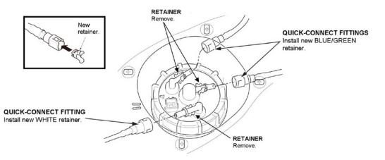
50. Connect the quick-connect fittings to the fuel tank unit.
