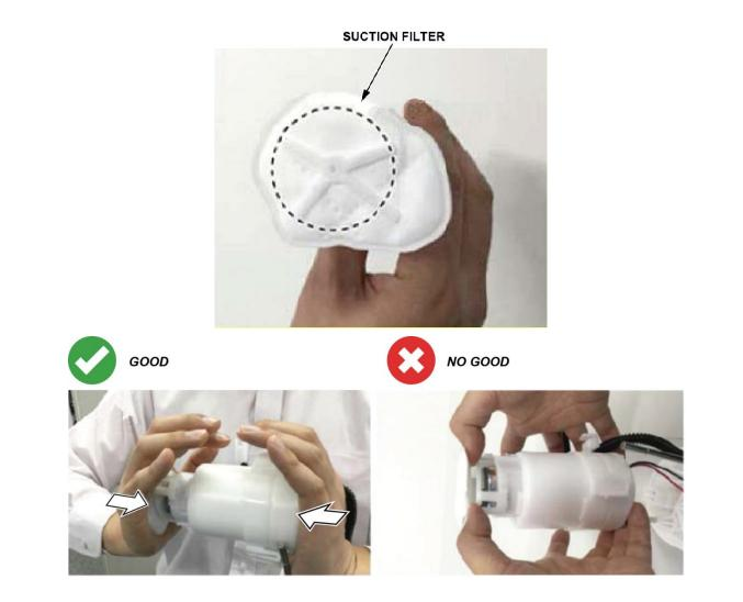
39. Install the fuel filter assembly to the reservoir.
