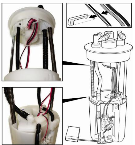
43. While compressing the fuel tank unit, make sure the movement is smooth and the fuel tube and wiring harness do not stretch, pinch, or bind.
