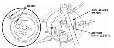
48. If the marks do not line up, friction between the fuel tank unit and the locknut may cause the fuel tank unit to turn while tightening. Observe the difference (shaded area), and loosen the locknut until the fuel tank unit can be rotated. Rotate the fuel tank unit **counter-clockwise** by the same amount, and repeat the tightening process.
