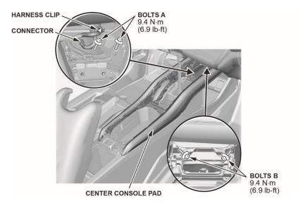
14. Remove the center console pad, and disengage the brackets from the bolts.
