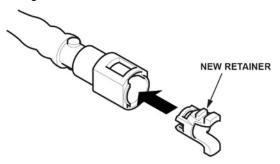
41. Connect the fuel line quick-connect fitting.
