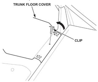
11. Open the trunk lid, then remove the trunk floor cover.
