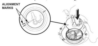
38. Press down on the fuel tank unit while turning the locknut clockwise by hand.
