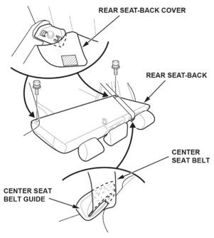
9. Pull out the center seat belt through the center seat belt guide and remove the rear seat-back.
