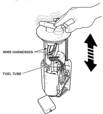
36. Install the new O-ring to the fuel tank, then partially install the new fuel tank unit.
