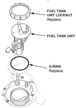
17. Prepare the fuel pump and parts to be replaced.
