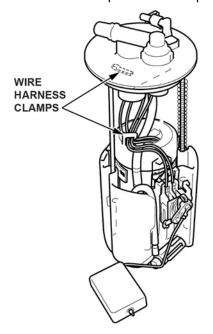
19. Press the tab on the fuel level sensor to release the lock. Then, push up on the fuel level sensor.
