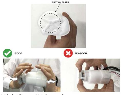
30. Install the fuel filter assembly to the reservoir:
