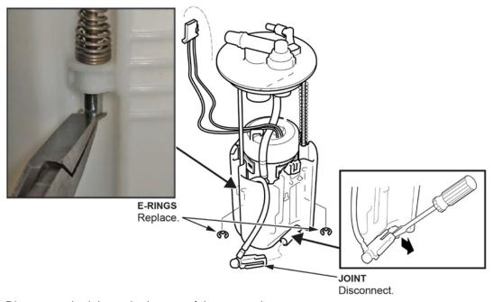
22. Disconnect the joint at the bottom of the reservoir.
