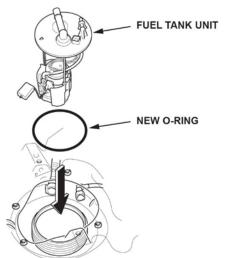
37. Line up the mark on the fuel tank unit to the marks on the fuel tank, then insert the fuel tank unit into the fuel tank.
