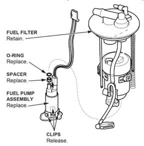
25. Pull the fuel pump assembly out of the fuel filter.
