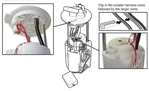
35. While compressing the fuel tank unit, make sure the movement is smooth and the fuel tube and wiring harness do not stretch, pinch, or bind.
