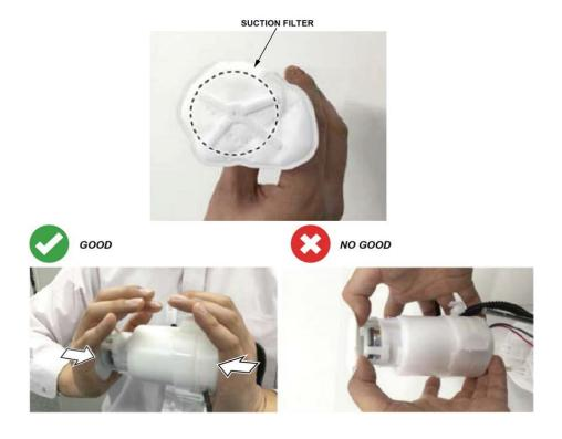
46. Install the fuel filter assembly to the reservoir.
