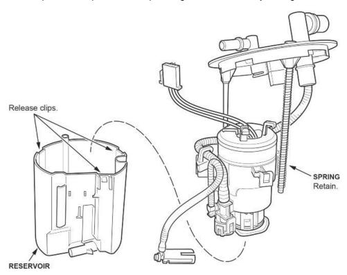
41. Release the three clips at the base of the fuel pump assembly and remove it from the fuel filter.
