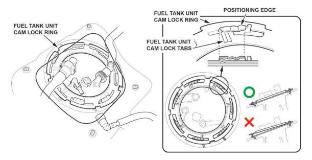
59. Tighten the fuel tank unit cam lock ring by turning clockwise using the fuel sender wrench.
