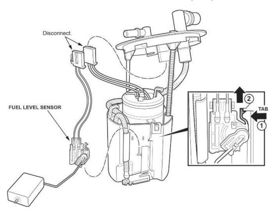
37. Disconnect the fuel level sensor harness and remove the fuel level sensor from the fuel tank unit.
