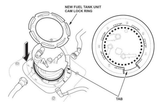
57. Connect the fuel vent tube and fuel tank vapor recirculation tube by slightly turning the fuel tank unit counterclockwise.
