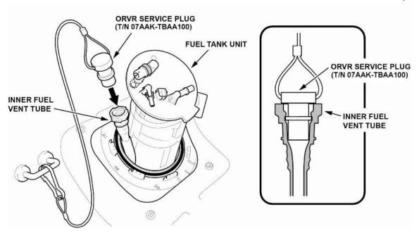
31. Install the ORVR service plug to the inner fuel vent tube. Make sure the ORVR service plug is fully seated by holding the inner fuel vent tube and gently pulling on the plug's lanyard.
