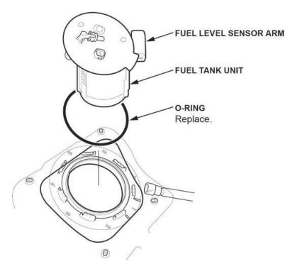
34. Prepare the fuel tank unit and parts to be replaced.
