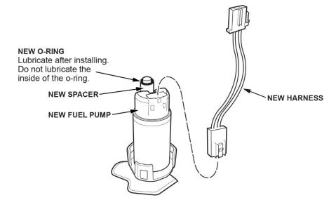
45. With the palm of your hand press the fuel pump into the suction fuel filter.
