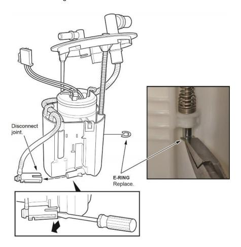
39. Disconnect the joint at the bottom of the reservoir.
