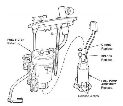
42. Install the new spacer onto the new fuel pump motor.
