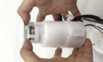
37. Install the fuel filter assembly to the reservoir.
