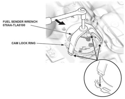
18. Turn the fuel tank unit cam lock ring counterclockwise to unlock it.
