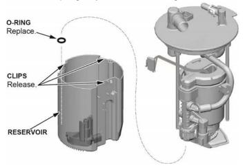
31. Release the three clips at the base of the fuel pump assembly and remove it from the fuel filter.
