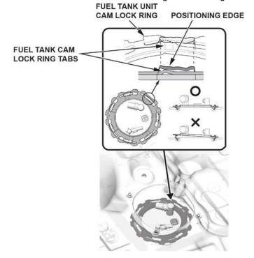
49. Tighten the fuel tank unit cam lock ring by turning clockwise using the fuel sender wrench.
