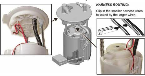
41. While compressing the fuel tank unit, make sure the movement is smooth and the fuel tube and wiring harness do not stretch, pinch, or bind.
