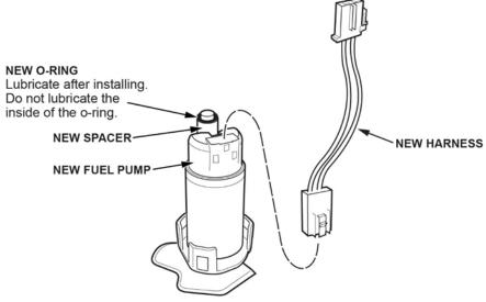
36. With the palm of your hand, press the fuel pump into the suction fuel filter.
