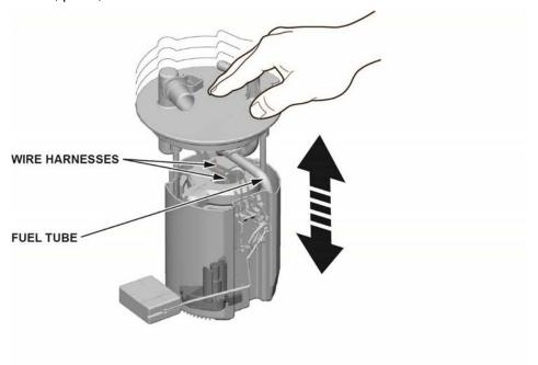
42. Install the fuel tank unit into the fuel tank with a new O-ring.
