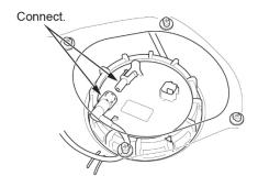
40. Connect the fuel tank unit connector.
