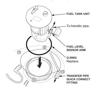
34. Line up the mark on the fuel tank unit to the marks on the fuel tank, then insert the fuel tank unit into the fuel tank. NOTE: To avoid any leaks, check the O-ring, either visually or by hand, to make sure it is not pinched.
