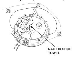
11. Remove the fuel tank unit locknut using the fuel sender wrench (T/N 070AA-T0AA100) as shown.
