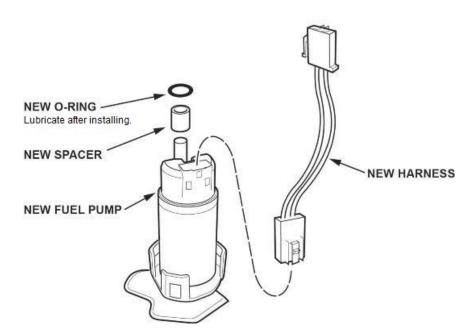
27. With the palm of your hand press the fuel pump into the suction fuel filter.
