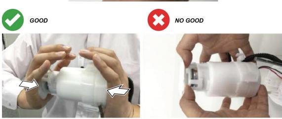
28. Install the fuel filter assembly to the reservoir.
