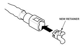
39. Connect the fuel line quick-connect fitting.
