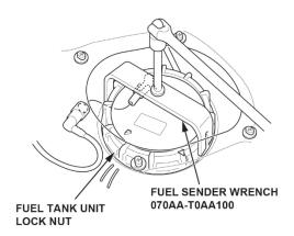
12. Remove the fuel tank unit.
