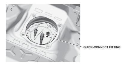
42. Connect the fuel tank unit connector.
