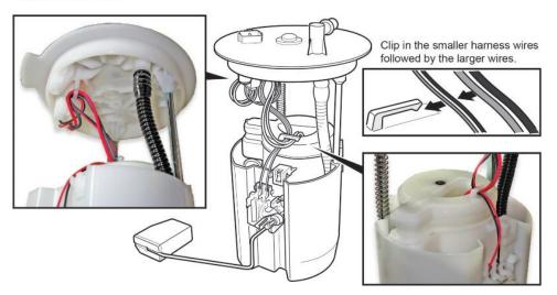
35. While compressing the fuel tank unit, make sure the movement is smooth and the fuel tube and wiring harness do not stretch, pinch, or bind.
