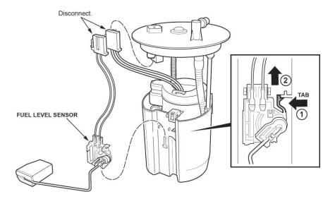
22. Disconnect the fuel level sensor harness, and remove the fuel level sensor from the fuel tank unit.
