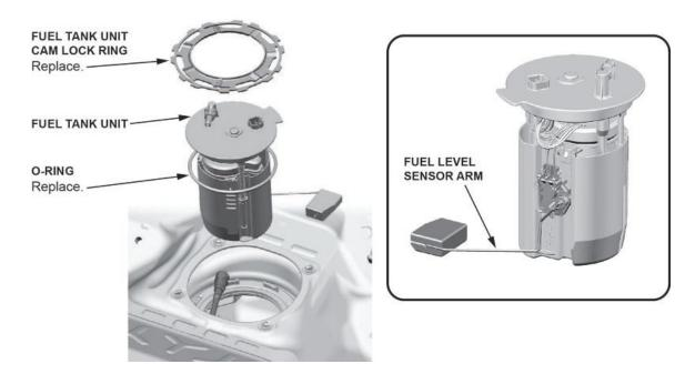
19. Prepare the fuel pump and parts to be replaced.
