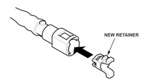
41. Connect the fuel line quick-connect fitting.
