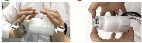
31. Install the fuel filter assembly to the reservoir.
