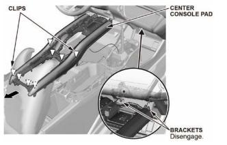
15. Remove the center console rear trim, and disconnect the connector.
