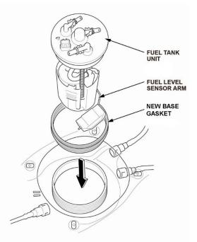
45. Line up the marks on the fuel tank and fuel tank unit as shown, then insert the fuel tank unit.
