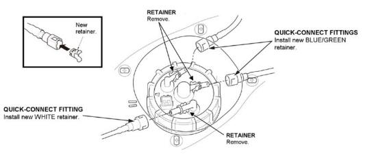
50. Connect the quick-connect fittings to the fuel tank unit.
