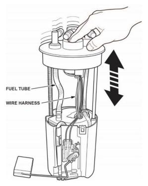
44. Partially insert the fuel tank unit into the fuel tank with a new base gasket.
