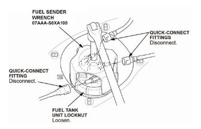
26. Remove the fuel tank unit locknut, then remove the fuel tank unit.
