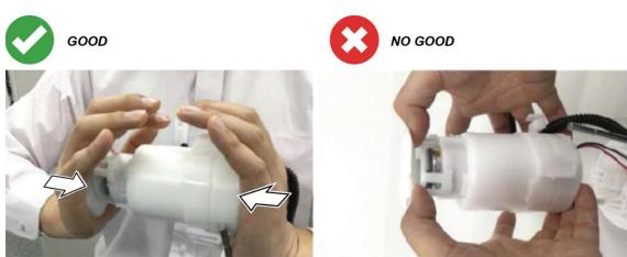
28. Install the fuel filter assembly to the reservoir.
