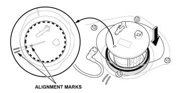
35. Align the mark on the new locknut to the start of the thread on the fuel tank.
