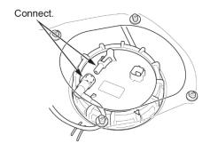
40. Connect the fuel tank unit connector.
