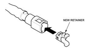
39. Connect the fuel line quick-connect fitting.
