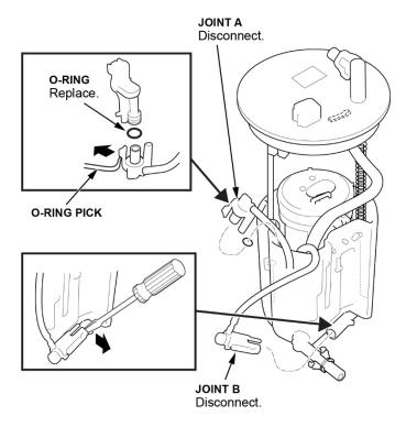
20. Disconnect joint B at the bottom of the reservoir.
