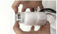
46. Install the fuel filter assembly to the reservoir.
