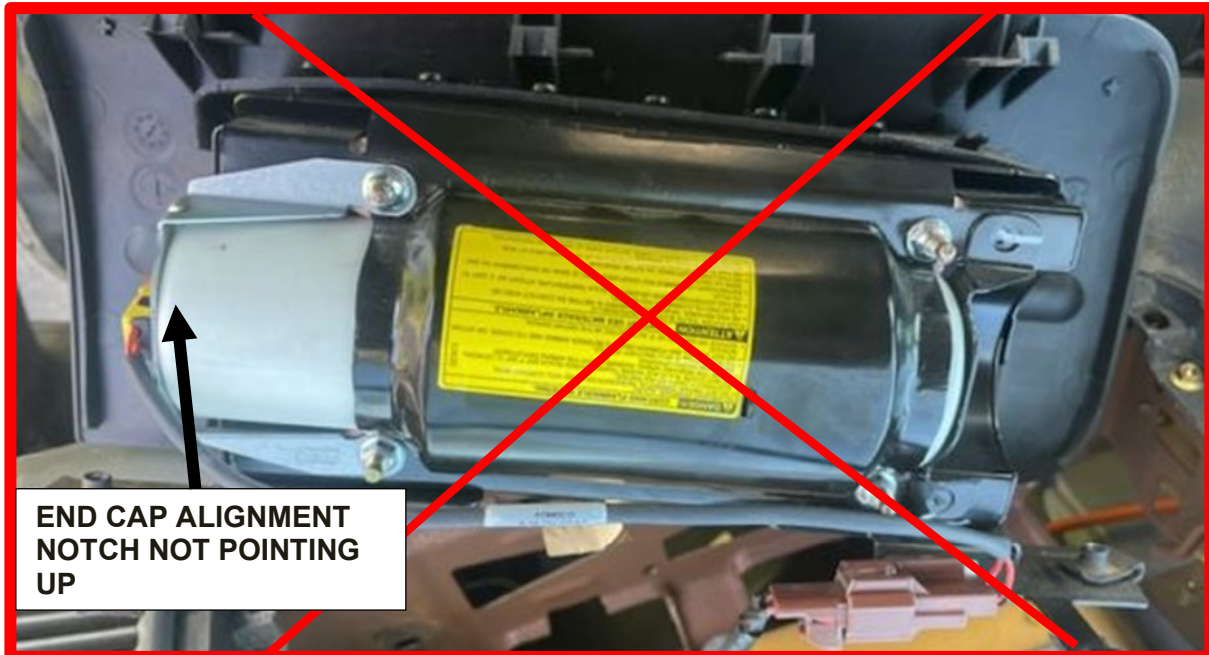
FIGURE 3 - INCORRECT ORIENTATION OF END CAP. ALIGNMENT NOTCH IS UPSIDE DOWN
