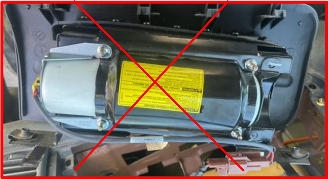
NO GOOD (NG) INCORRECT ORIENTATION OF END CAP
