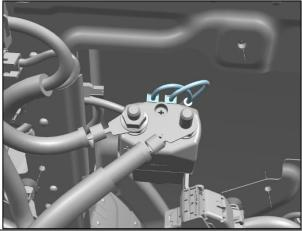
Note: Ensure the Relay Wires are in the correct position and not trapped before installing the terminal nut.
