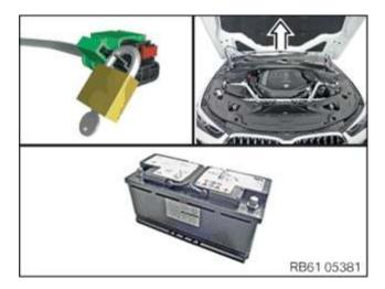
Deactivate the vehicle electrical system HV (if required) and 12V as described in the VIN specific repair instruction.
