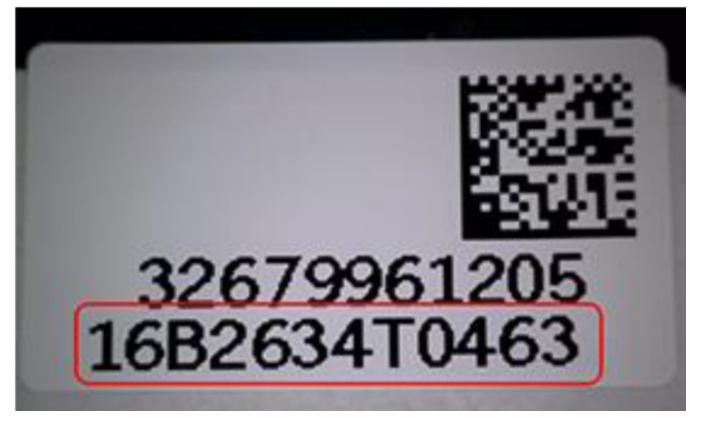
Before installing the replacement part, the new air bag module's serial number (circled above) must be documented by the technician on the repair order so it can also be entered into the warranty claim's comment section.
