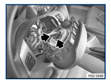
REP-REP-RAF1532-3234030 Removing and installing/replacing airbag unit (sport steering wheel), VIN: XXXXXX
