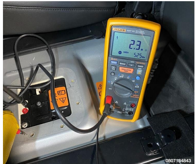
Figure 38 – Measure and Record Isolation Resistance Between HV Negative Test Point and Chassis Ground
