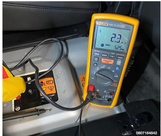
Figure 37 – Measure and Record Isolation Resistance Between HV Positive Test Point and Chassis Ground
