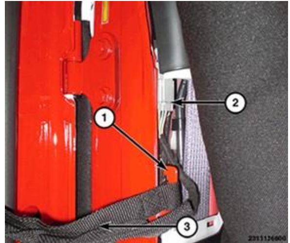
Figure 20 – Harness to Support Bracket
