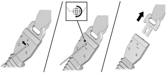
8. Disconnect the driver's and/or passenger's side seat belt outer lap tensioner connector from the floor wire harness.
