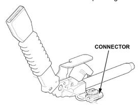
9. Remove the pretensioner mounting bolt, then remove the pretensioner.
