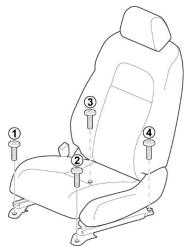
2. Move the driver's and/or passenger's front seat to the forwardmost position and remove the rear seat bolts.
