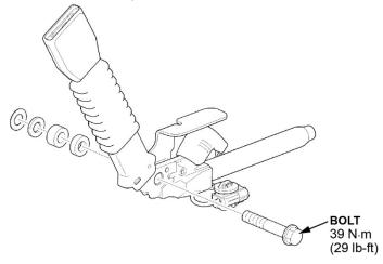
10. Install the new pretensioner and torque the bolt to 39 N·m (29 lb-ft).
