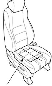
The weight must be placed precisely on the center line of the seat.
