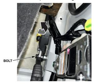
7. Use a small screwdriver to release the seat belt from the quick connector.
