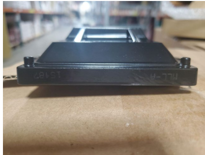
Image 4-1: Replacement Module with etched “A” marking
