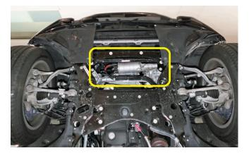
1. Raise vehicle on lift to access the steering gear (circled) beneath the vehicle.
