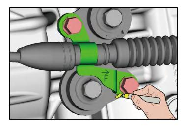
**STEP 13:** Remove the two retaining bolts and remove the cable bracket.
