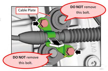
**STEP 14:** Remove the gear selector cable and shifter arm together from the shifter arm shaft.
