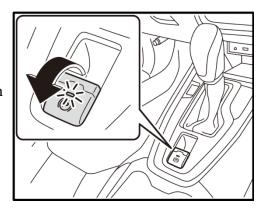
**STEP 2:** Using a plastic trim tool, remove the rubber pad located in front of the gear selector.
