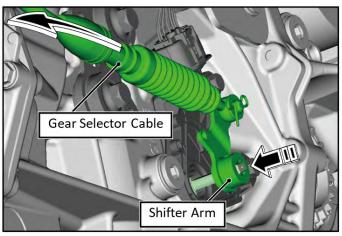
**STEP 20:** Install the cable bracket using the alignment marks made in Step 13. Torque the mounting bolts to 18Nm (13ft-lbs.).
