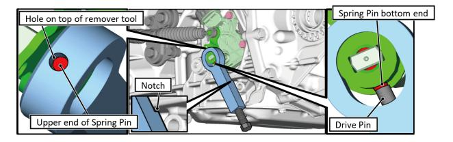
STEP 10: Using HAND TOOLS ONLY, tighten the threaded portion of the removal tool until the spring pin is fully removed. Discard the spring pin once it is fully removed. DO NOT reuse the spring pin.
