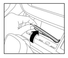
**STEP 3:** Insert a small screwdriver into the round hole located under the rubber pad. This will release the gear selector lock. Move the gear selector into the Neutral position.
