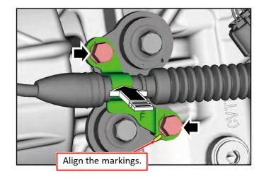
**CAUTION: DO NOT** install the cable bracket in the opposite position. Doing so will damage the gear selector cable.
