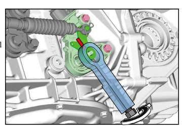
**STEP 12:** Using a marker or paint pen, make an alignment mark on the cable bracket and cable plate as show in the right image. This mark will be utilized in further steps.
