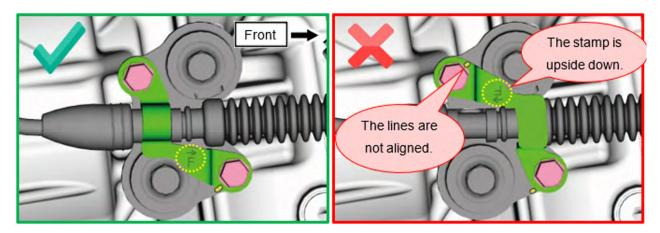
**STEP 21:** Align the shifter arm hole and the shaft hole.
