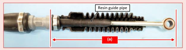
If the resin guide pipe is damaged, the inner cable can become slackened when operating the gear selector lever and the shifter arm become inoperative. As a result, the shift positions of the gear selector lever and the inhibitor switch do not match, causing malfunctions such as an engine no crank/no start condition.
