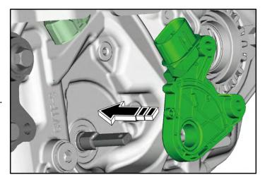
**STEP 18:** Connect the electrical connector. Install the two mounting bolts hand tight only. The bolts will be torqued after a final adjustment is made.
