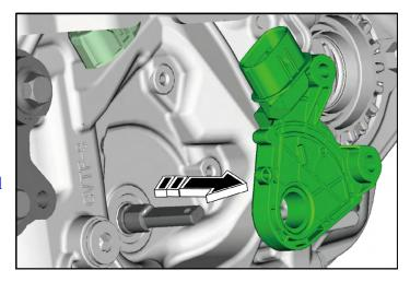
**STEP 17:** Install the new inhibitor switch. Maintain proper alignment with the shifter arm shaft. Refer to Work Tips Video at 01:33.
