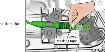
**STEP 24:** Remove the masking tape from the gear selector cable.
