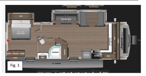
Figure 2 shows a 27RK White Hawk (4G) floorplan. Inspect the 48 x 36 window, shown by the red arrow. Proceed to the instructions if window has an exit window sticker and or red handle and red screen knob.
