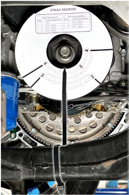
ZIP TIE Attach a zip tie to the frame and line up as shown.
