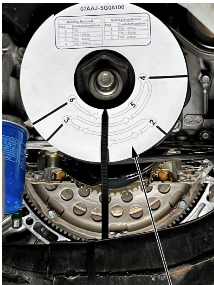
ZIP TIE Attach a zip tie to the frame and line up as shown.
