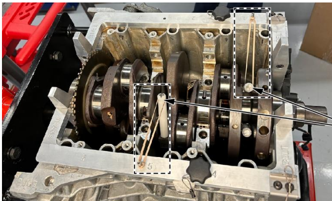
TIE DOWNS Make sure the tie downs are attached to cylinders 1 and 5.
