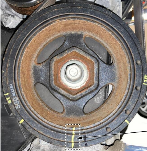
CRANKSHAFT PULLEY Mark with a vertical line from the 6 o'clock position.
