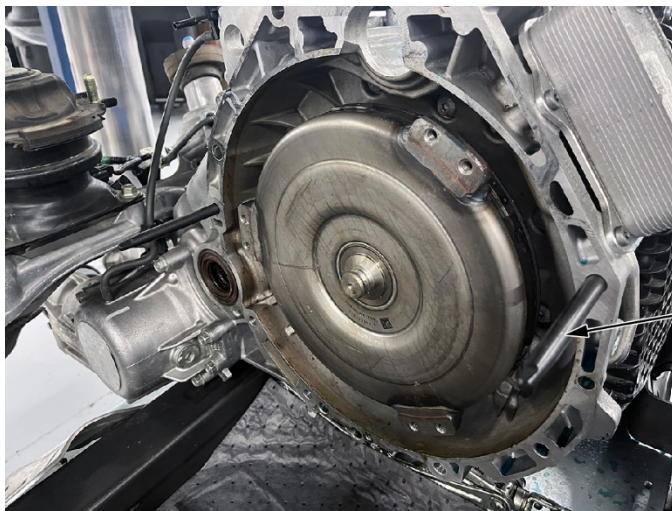
TRANSMISSION ALIGN PIN P/N 07AGG-5J4A100
