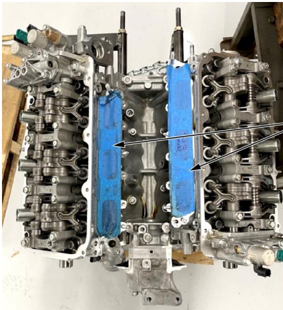
PAINTERS TAPE Apply tape to the intake ports.
