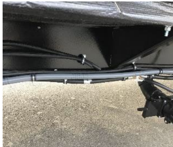
REFERENCE OF FLEXIBLE CONDUIT ROUTING ON I-BEAM
