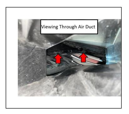
c) Turn the air duct so that the upper driver's side bumper cover claws can be viewed by peering through the tube with a flashlight.
