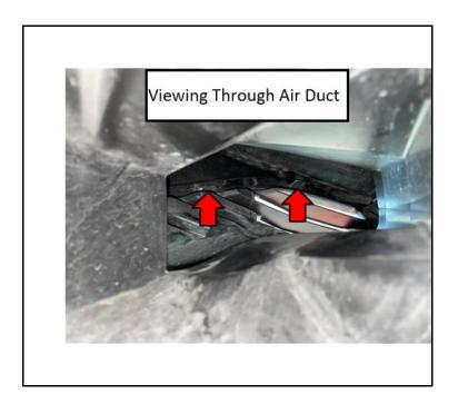
c) Turn the air duct so that the upper driver's side bumper cover claws can be viewed by peering through the tube with a flashlight.
