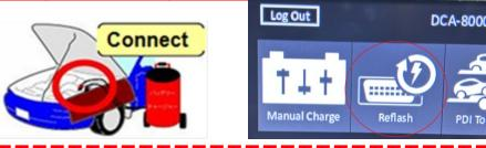
NOTE: Make sure that HV charging cable is not connected to HV battery charging port.
