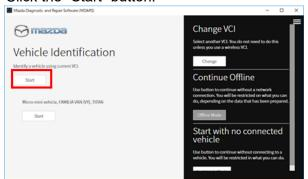
2. The Vehicle Identification process will start and automatically inspect every connection and then collect the vehicle information.
