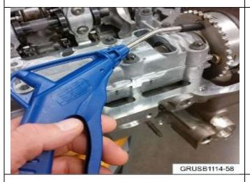
5. Clean the threads on the VANOS assembly using compressed air to remove the excessive oil.
