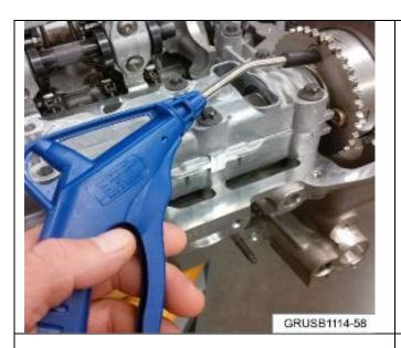
11. Clean the threads on the VANOS assembly using compressed air to remove the excessive oil.
