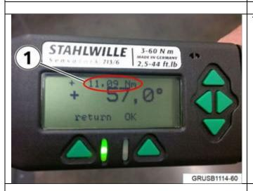
While performing the angle torque the digital screen on the torque wrench will display the current Nm meter value. This value should be between 8 Nm – 14 Nm.
