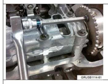
10. Turn the engine by hand using a suitable wrench on the crankshaft central bolt to align the bolt (1) with as shown in the illustration.
