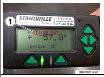
Note: The tool will be on a slight angle when Tightening.
