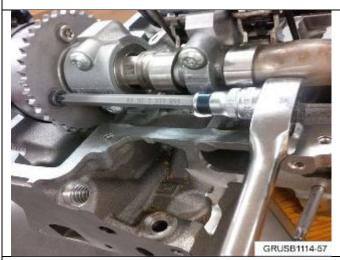
4. Turn the engine by hand using a suitable tool on the crankshaft central bolt to align one of the bolts (1) as shown in the illustration.
