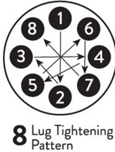
Figure 4 - Lug Tightening sequence
