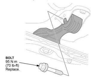
13. Attach the subframe adapter to the front subframe.
