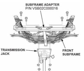
14. Raise a transmission jack and line up the slots in the subframe adapter arms with the bolt holes on the transmission jack base, then securely attach the four bolts. Then, remove the bolts highlighted in yellow only.
