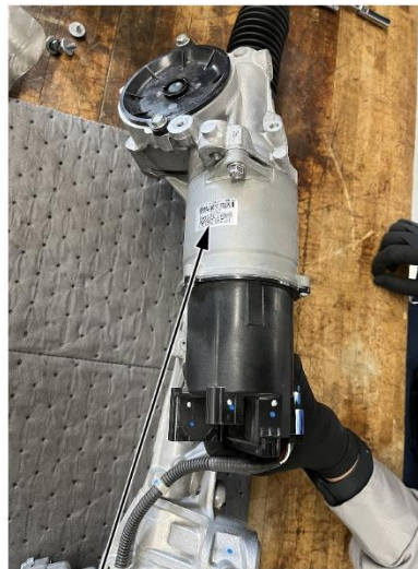
BARCODE Install with barcode facing up.
